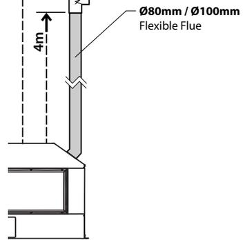
**Vertically Terminated Internally:** (utilizes the escea internal vertical power flue enclosure kit)
